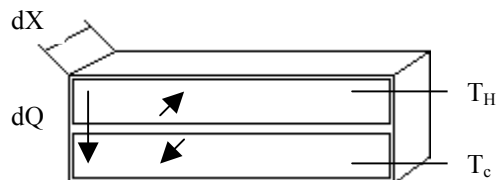
Figure 8 rectangular heat exchanger, Plate_HE, model physical layout
