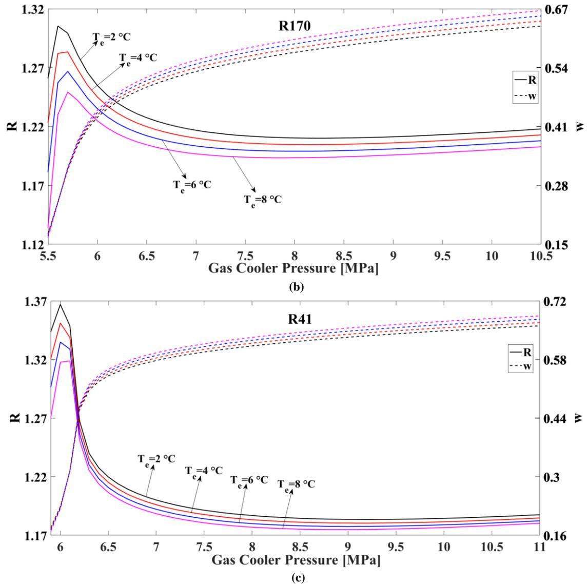
**Figure 8.** Effects of the evaporator temperature based on the gas cooler pressure on the optimum performance improvement ratio and entrainment ratio for R744 (a), R170 (b), and R41 (c).
