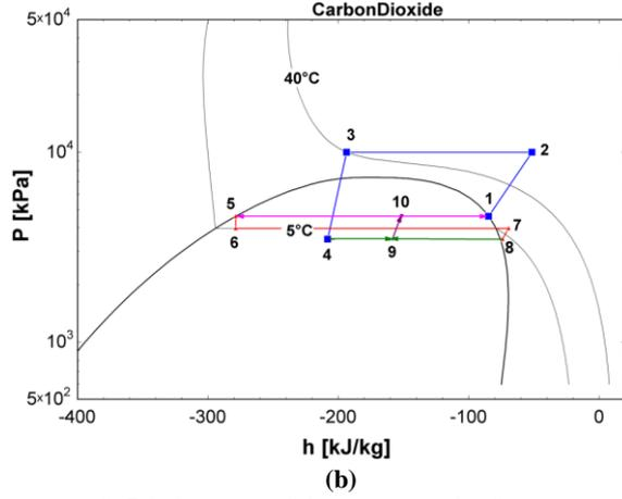
**Figure 2.** P-h diagrams of the transcritical refrigeration cycle (a) and the EERC including constant pressure mixing (CPM) ejector (b) for CO<sub>2</sub> (Klein, 2017).
