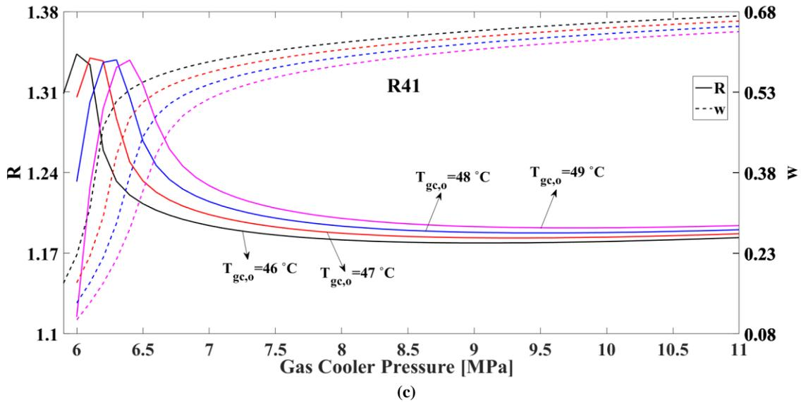
**Figure 7.** Effects of the gas cooler outlet temperature based on the gas cooler pressure on the optimum performance improvement ratio and entrainment ratio for R744 (a), R170 (b), and R41 (c).
