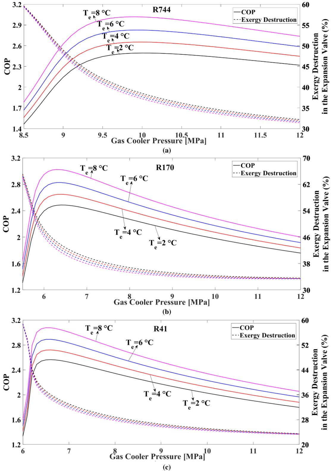
Figure 5. Effects of the evaporator temperature on the performance and percentage expansion losses for R744 (a), R170 (b), and R41 (c) with respect to the gas cooler pressure.
