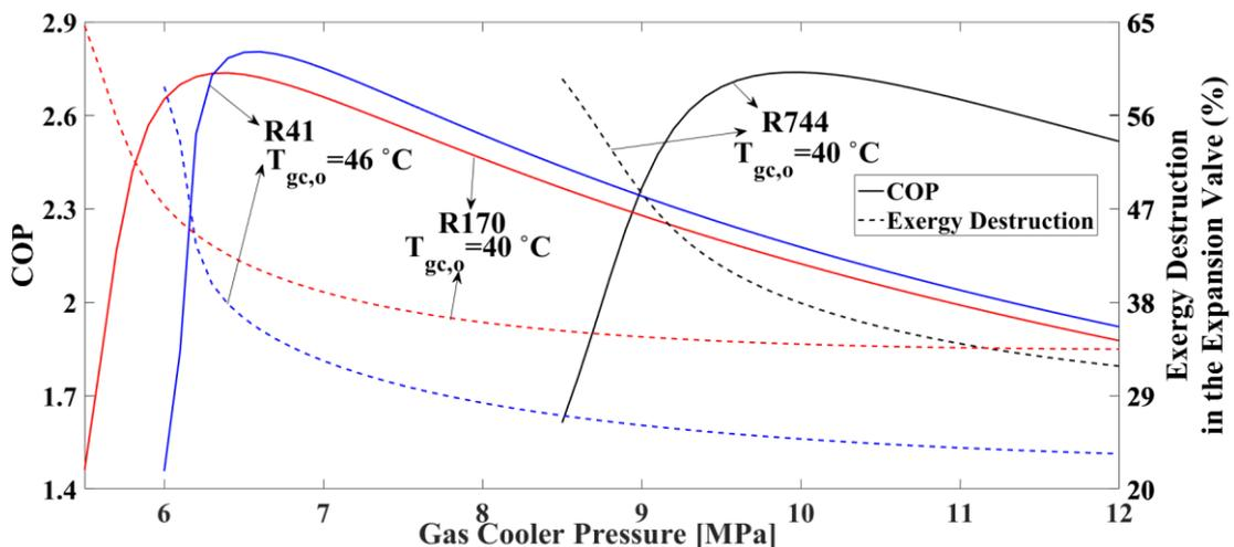
**Figure 4.** Comparisons of the COP, percentage expansion losses, and gas cooler pressure of the highest performance point for R744, R170, and R41 with respect to different gas cooler outlet temperatures at which they perform their highest performance.
