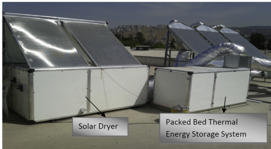
Fig. 2. Assembly drawing of solar dryer and packed bed thermal energy storage system.
