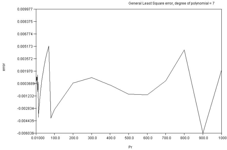
$$\left. \frac{\partial \theta}{\partial y} \right|_{y=0} = \theta' = a_0 \Pr^{1/4} + a_1 \Pr^{1/2} + a_2 \Pr^{3/4} + a_3 \Pr$$
