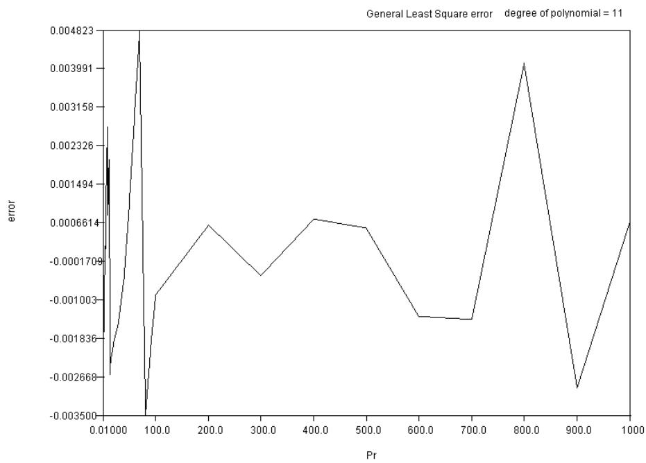
$$\left. \frac{\partial \theta}{\partial y} \right|_{y=0} = \theta' = a_0 \Pr^{1/4} + a_1 \Pr^{1/2} + a_2 \Pr^{3/4} + a_3 \Pr + a_4 \Pr^{5/4} + a_5 \Pr^{3/2} + a_6 \Pr^{2/4} + a_7 \Pr^2$$
