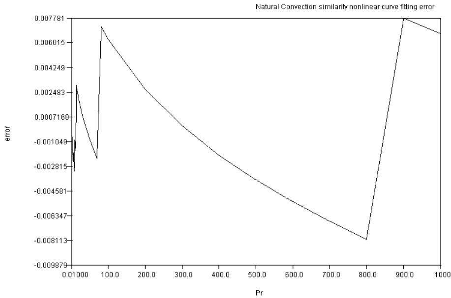
As it is seen from the results, error level of this equation is one order better than the Incropera equation. Error level can be further reduced in nonlinear equations by increasing number of terms as well. Let us assume the equation in the form of
